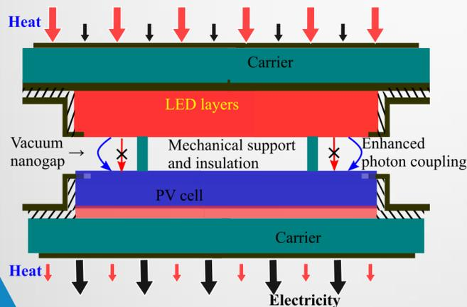
In TPX-POWER we investigate if reaching practical energy harvesting applications using thermophotonics is feasible with presently available and emerging technologies. To this end, we aim to demonstrate TPX power generation in an integrated device to validate its potential for next generation thermal energy harvesting at low-to-medium temperatures.
