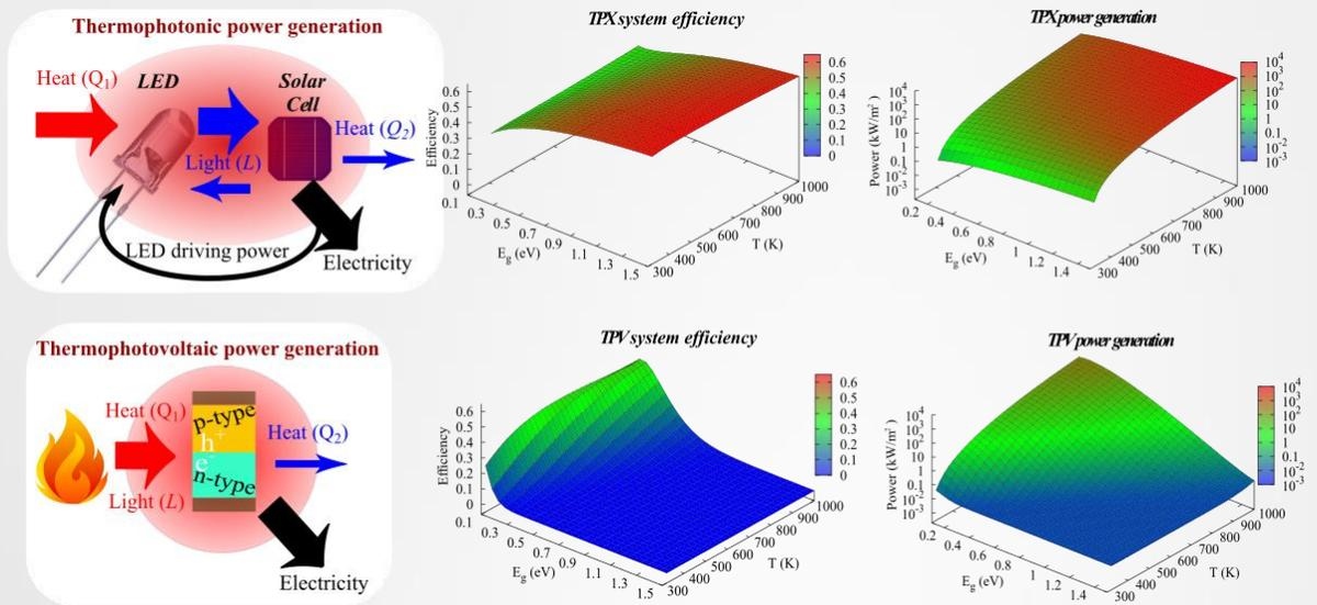
Figure: Schematic comparison of the basic principles and performance of a thermophotonic (TPX) and thermophotovoltaic (TPV) heat engines. Under ideal conditions the TPX system can operate at very high system efficiencies and powers over a broad range of temperatures and material bandgaps, whereas TPV systems typically require very small bandgap materials and high temperatures.
